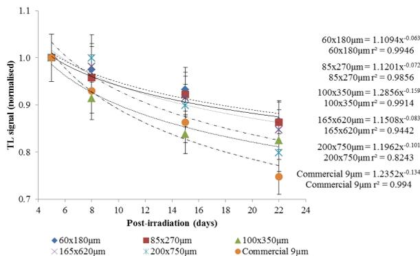
Figure 4. Post-irradiation fading for fabricated Ge-doped flat fibres and also commercial fibres under normal ambient conditions
